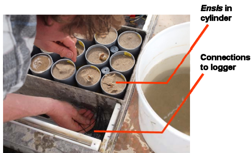
Figure 4. Placement of sediment cores with live Ensis connected to a valve monitor in one of the trays which are mounted on the lander.
