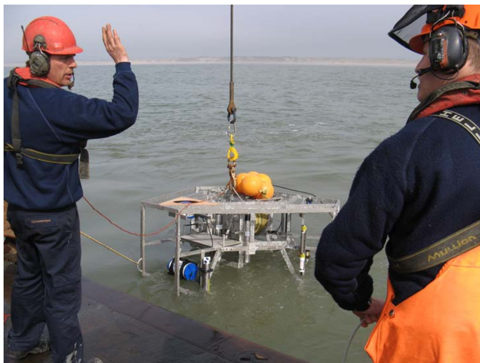
Figure 7. . Deployment of one of the lander platforms off the coast of Egmond.
