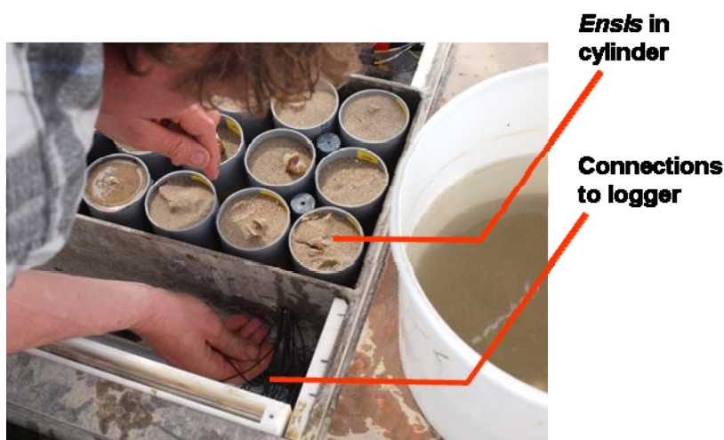
Figure 6. Placement of sediment cores with live Ensis connected to a valve monitor in one of the trays which are mounted on the lander.
