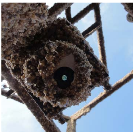
Figure 49. Overgrown Alec Turbidity sensor. The wiped area is perfectly clean while the surrounding area is heavily over grown by barnacles.
