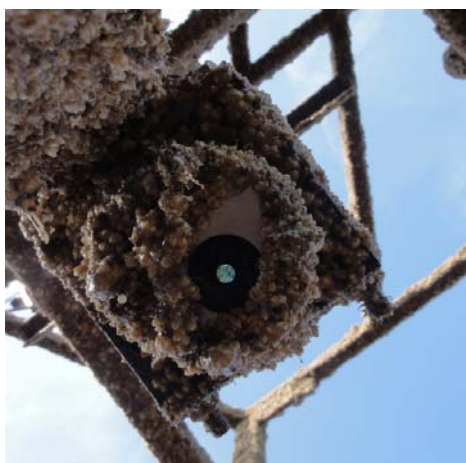
Figure 58. Overgrown Alec Turbidity sensor. The wiped area is perfectly clean while the surrounding area is heavily over grown by barnacles.
