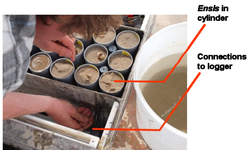
Figure 6. Placement of sediment cores with live Ensis directus connected to a valve monitor in one of the trays which are mounted on the lander.
