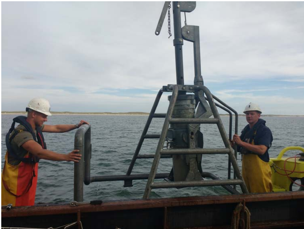
Figuur 6: Reineck box-corer (foto Jack Perdon).
